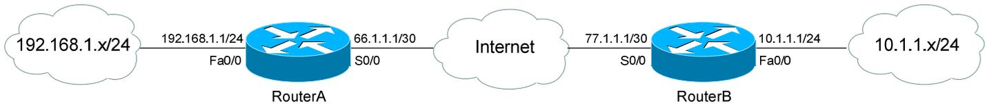
**Generic Routing Encapsulation (GRE)** is a tunneling protocol that does *not* perform security functions, such as encryption or hashing.
