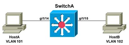
Configuring inter-VLAN routing using SVIs is very simple. First, the VLANs must be created:
